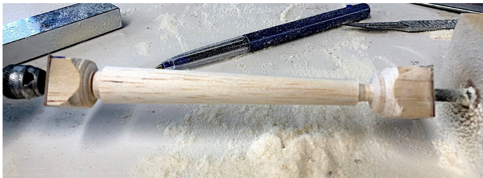
Above: Production of a mandrel for the tail boom turned in White Oak.
